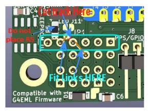
A surface mount 2x8 header (J5) is required for the LMX2575 (#6). This fits directly below the RP2040 Zero. At the time of writing, Lehane G8KMH is testing his revised firmware to support these PLLs before publishing it.
