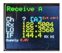
When he desired channel is reached, a press on the **Enter** button will assert channel control and return the display to 'monitoring mode'. If **Enter** is not pushed, this happens after 5 seconds.
